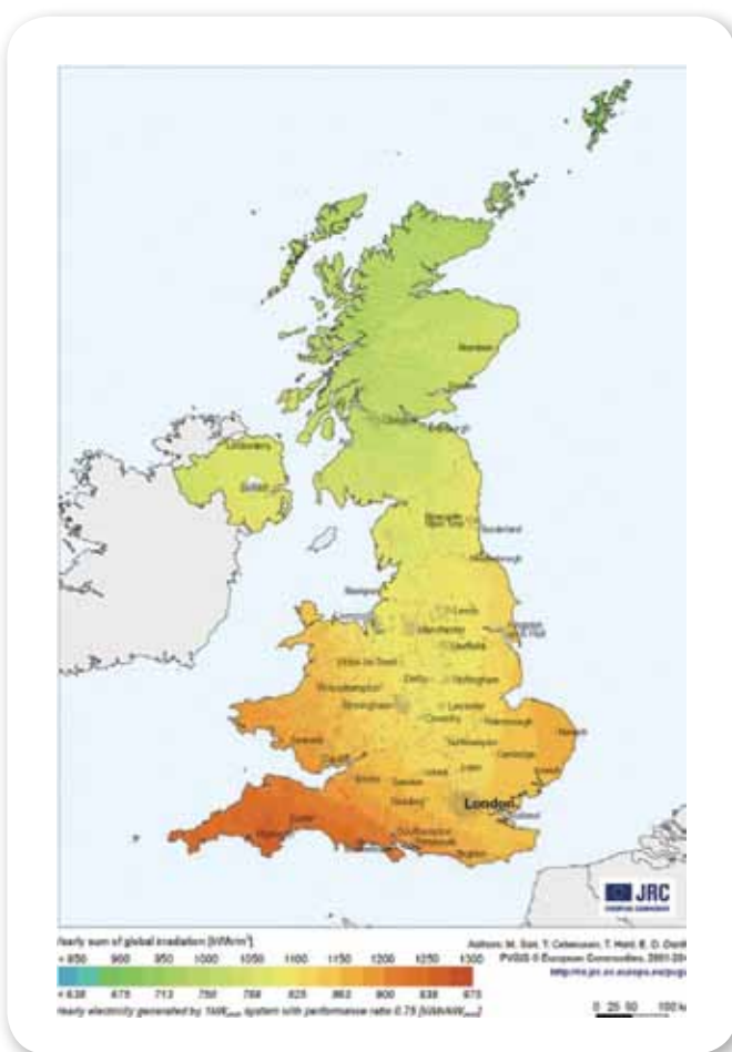
Figure 5. Map of UK and Republic of Ireland Solar Irradiation (PVGIS © European Communities, 2001-2008)
